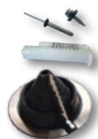
The weather-resistant, easy-to-install pipe collar with seal can be used to insert insulated solar piping through the roof. The scope of delivery includes bulb-tite rivets for corrugated cement asbestos and drilling screws for installation on all sheet metal roofs, plus sealing compound in a practical application cartridge and installation instructions.
